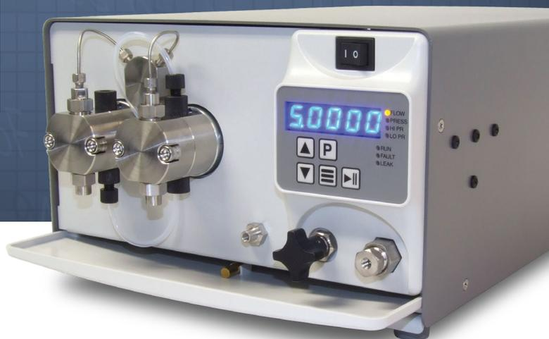
The high performance CP Class consists of dual-headed, positive displacement piston pumps with constant pressure control, covering a wide range of flows, with pressures up to 25,000 psi. Standard fluid path materials are Stainless Steel, with optional Titanium and Hastelloy also available. Other optional features include jacketed pump heads for temperature-controlled applications.
